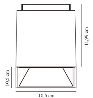
Voltage (V): 230 Volt IP degree: IP20 Maximum bulb wattage (W): 50W Class (Class 1, Class 2, Class 3): Class 2 (Double isolated) Socket type: GU10 Parallel connection: True
